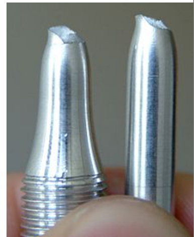
Fig. 3 Tensile test of AlMgSi alloy
