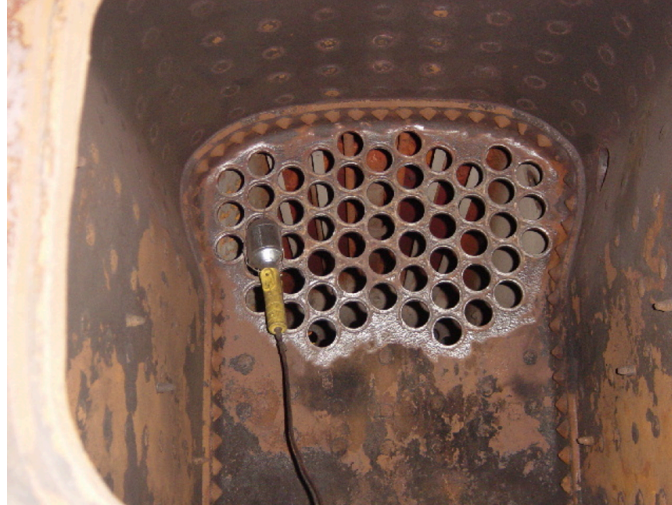
Fig. 6 Rear flue sheet.
